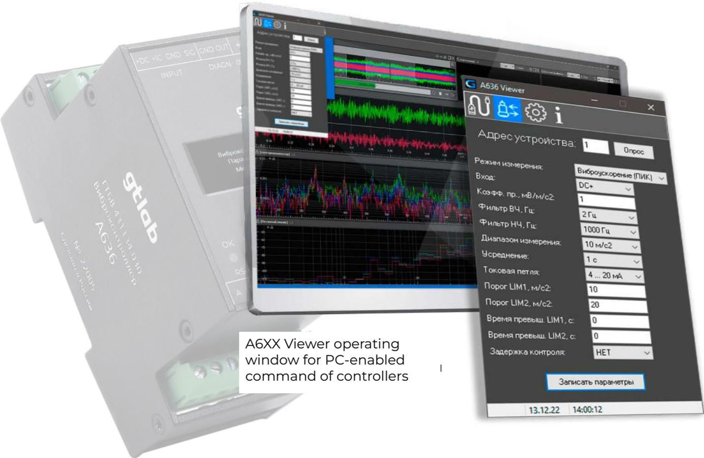
A6XX Viewer operating window for PC-enabled command of controllers
