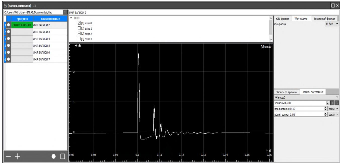
Playback of signals with the possibility of selecting individual fragments for their subsequent spectral analysis.
